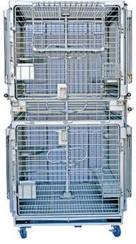
The vertical pairing cartridge feature is self contained, and can be removed. The top cage floor and waste pan telescope to the rear of the cage. This allows the waste in the top waste pan to flow to the rear trough. Latches secure the floor in place. A mid-section door on the front of the cage allows added security, and is used to lock a metabolic pan in place (optional).
